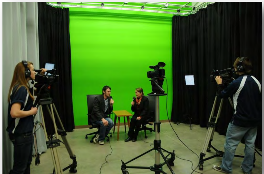
HDTV Production Studio set up for virtual set interview with two camera operators and one “locked down” wide-shot camera
